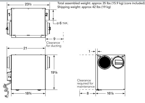
Clearance required for maintenance 16<sup>1</sup>/<sub>8</sub>
